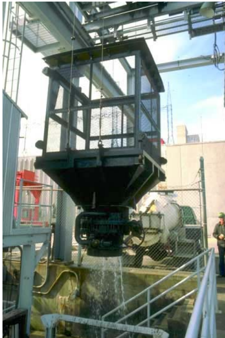
Photo 17: Transport facility at Mactaquac dam on the Saint John river (New Brunswick, Canada). (Photo Larinier)
