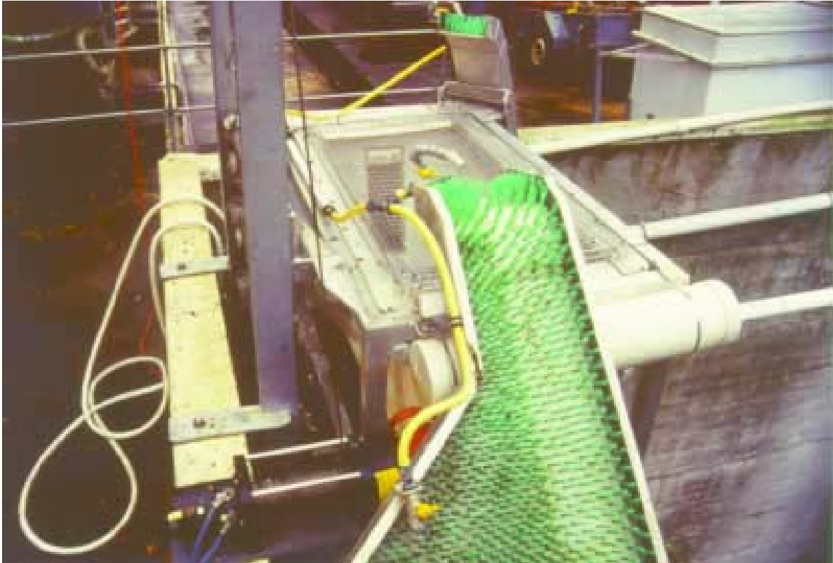
Photo 28: Elver trap at Karapiro dam (New Zealand). This floating trap is periodically raised to pass the small eels upstream. (Photo Larinier)
